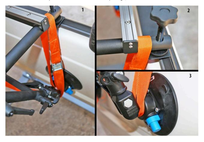
WARNING! The mounting procedure described above requires extreme care and must be carried out as written so as to avoid loss of grip of the suction cups, blocking levers or safety belts and consequent damage to persons or equipment: Geko is not responsible for damage due to incorrect mounting. For further details on the use and safety of the suction cups, see the Manfrotto manual included.
